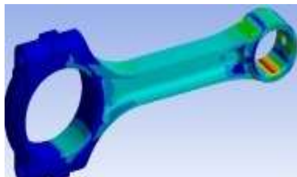
Fig.4 Structural analysis of connecting rod of a tractor -16
